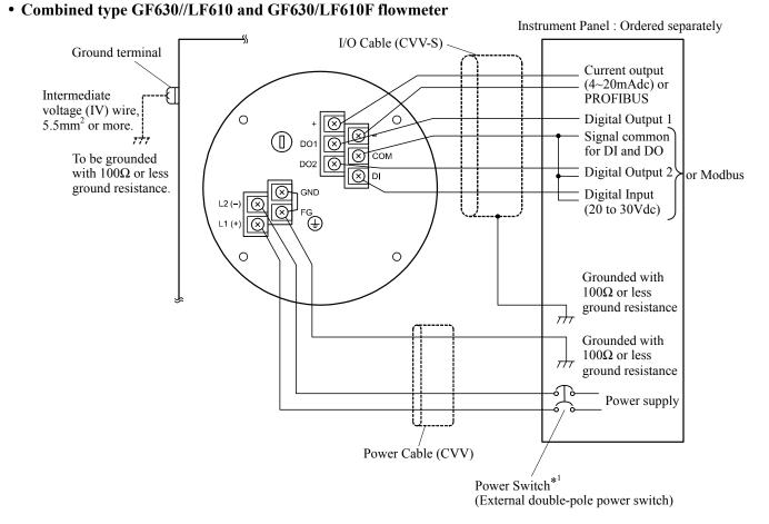
Figure 6. Combined type GF630/LF610 and GF630/LF610F flowmeters Wiring Diagram
