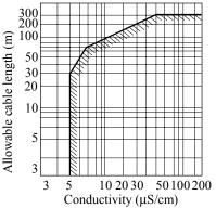
Figure 8. Electrical Conductivity and Cable Length
